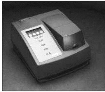
**Gambar 2.2** Spektrofotometer *Single Beam* (Yudhono, 2017)
