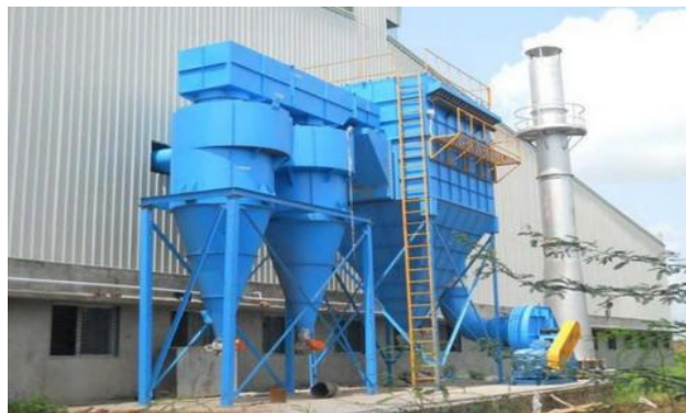
Gambar 2.7 Bag House Filter (Suryani et al., 2023)
