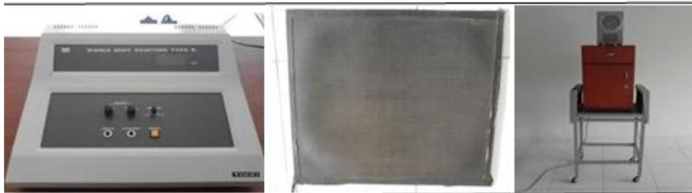
Gambar 26. *Chronoscope Digital*, Karpet Reaksi, Lampu Stimulus.
