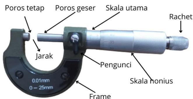
**Gambar 10.** Bagian-bagian Mikrometer Sekrup
