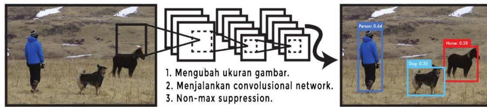
Gambar 7. Proses Sistem Deteksi YOLO (Redmon, dkk., 2016).
