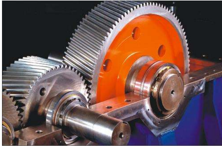
Gambar 2. 8 Helical Gear Box [9]
