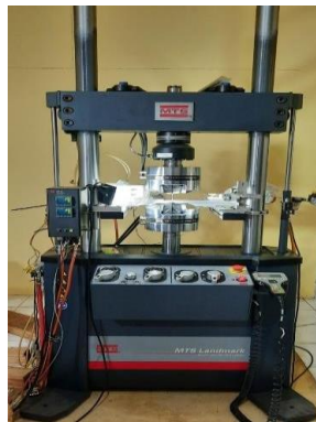
Gambar 12. Hydraulic servopulser mesin landmark MTS 100 kN.
