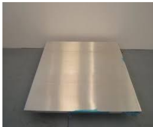
Gambar 8. Material magnesium AZ31B
