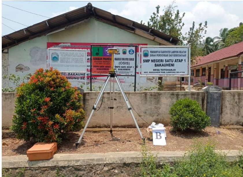
Gambar 18. Proses pengambilan data GPS.
