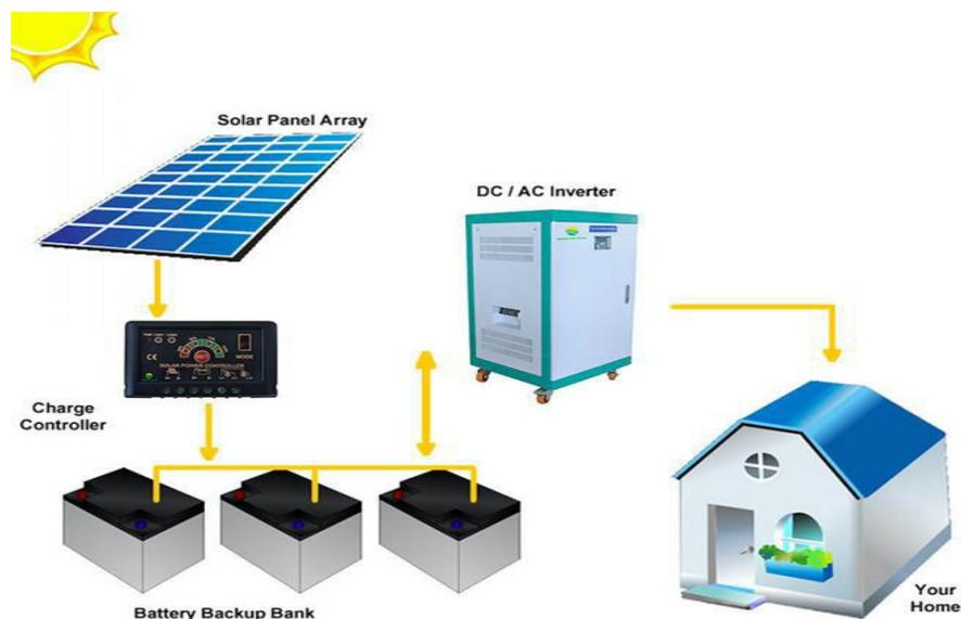
Gambar 2.2 Sistem PLTS *Off Grid* (Sumber:
