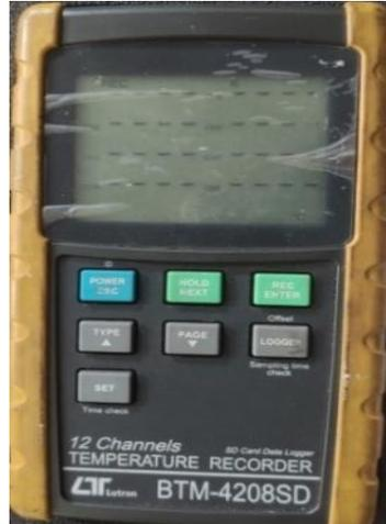
Gambar 3.2 *Temperatur Recorder Data logger*
