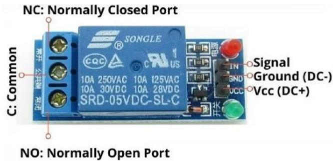
Gambar 2. 7 Relay 1 Channel
