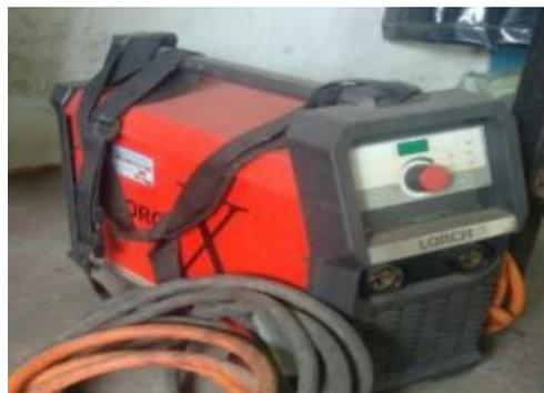
Gambar 3.2 Mesin Las SMAW (*Shielded Metal Arc Welding*)
