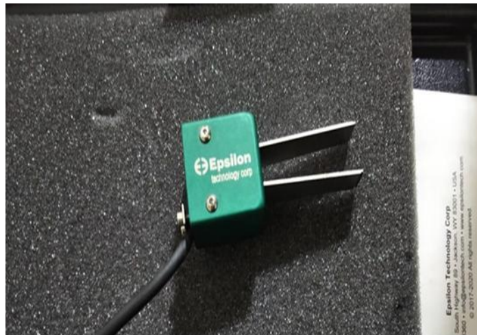
Gambar 3. 6 Clip Gage on Displacement (COD)
