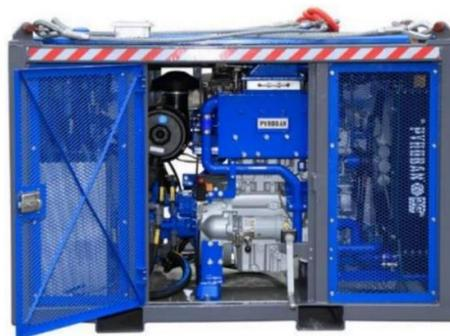
**Gambar 7.** Alat akuisisi *logging*, *Power pack* (Booz, 2017)
