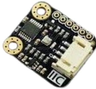
Gambar 2.7 Gravity BME280 Sensor [15]
