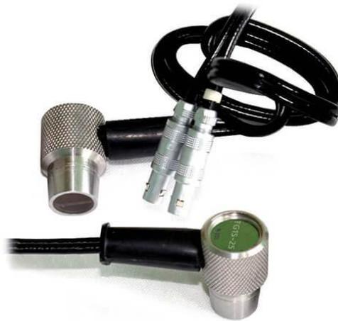
**Gambar 2. 9** Probe Dual Element
