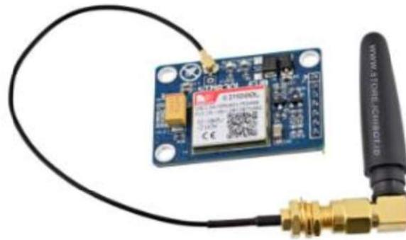
Gambar 2. 5 Modul GSM SIM800I V2
