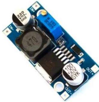
Gambar 2. 4 Modul LM2596 DC-DC Step Down
