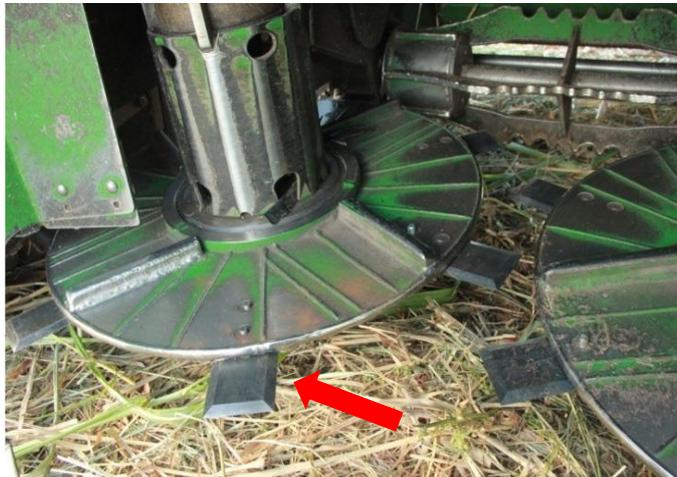
**Gambar 2.1** *Sugarcane Harvester Blades* (Ma et al., 2014)
