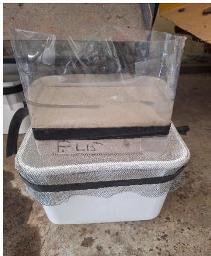
Gambar 4. Proses pengujian infiltrasi *paving block porous*.
