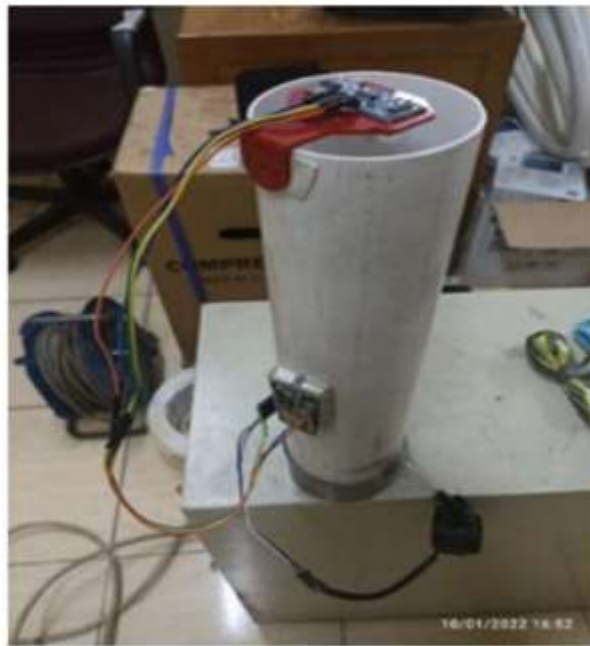
Gambar 2.8 Prototipe Sistem Monitoring Tangki Bahan Bakar Genset Peneliti Terdahulu (Wenas, 2021).
