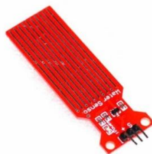
Gambar 2.8 Water Level Sensor
