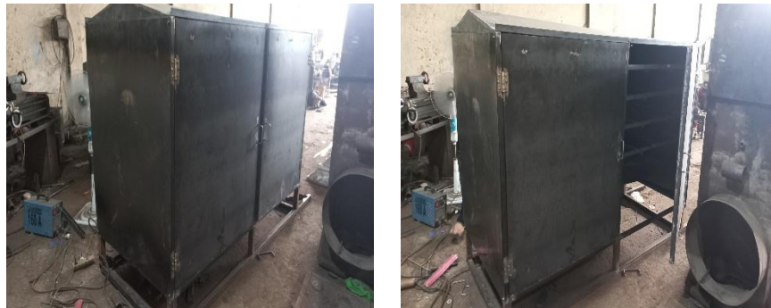
Gambar 3.5 Finishing penempelan dinding bed dryer .
