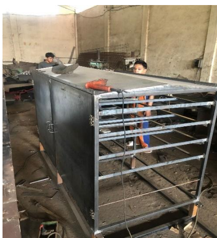
Gambar 3.4 Finishing penempelan dinding bed dryer
