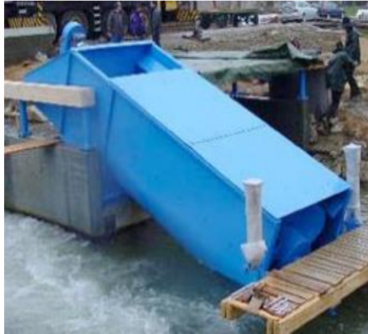
Gambar 2. 9 Screw Turbine Type Closed Compact Installation
