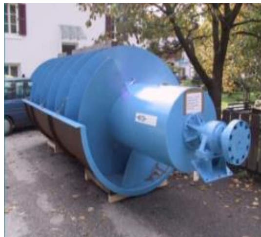
Gambar 2. 8 Screw Turbine Type Steel Trough ( Sumber : Karim dkk, 2023)
