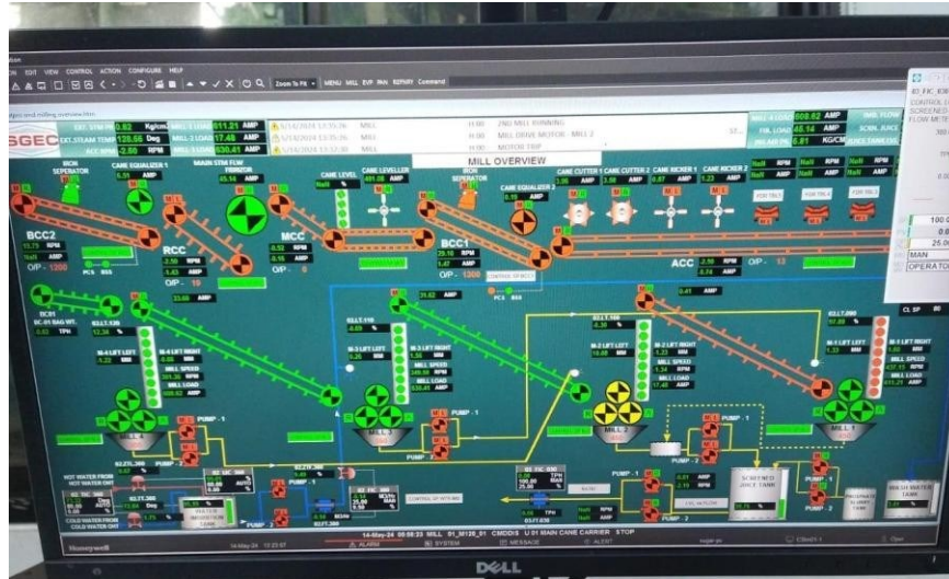
Gambar 2.1. Sistem kontrol terdistribusi (DCS) mill PT PNS
