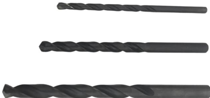
Gambar 3.3. Pahat Twist Drill HSS Diameter 4 mm, 6 mm dan 8 mm
