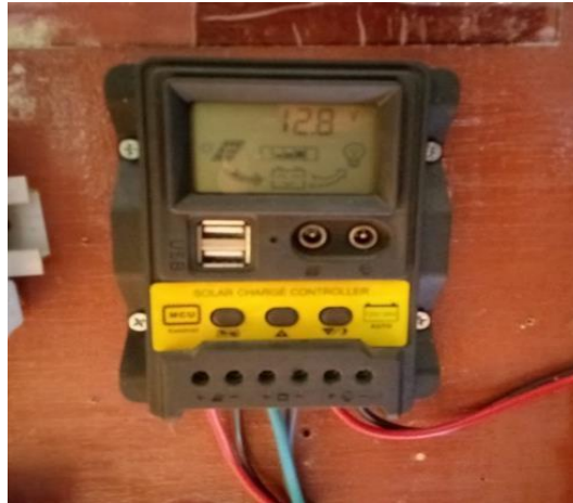
Gambar 11. Solar charge controller (PWM 12V/24V 30A - K-1688)
