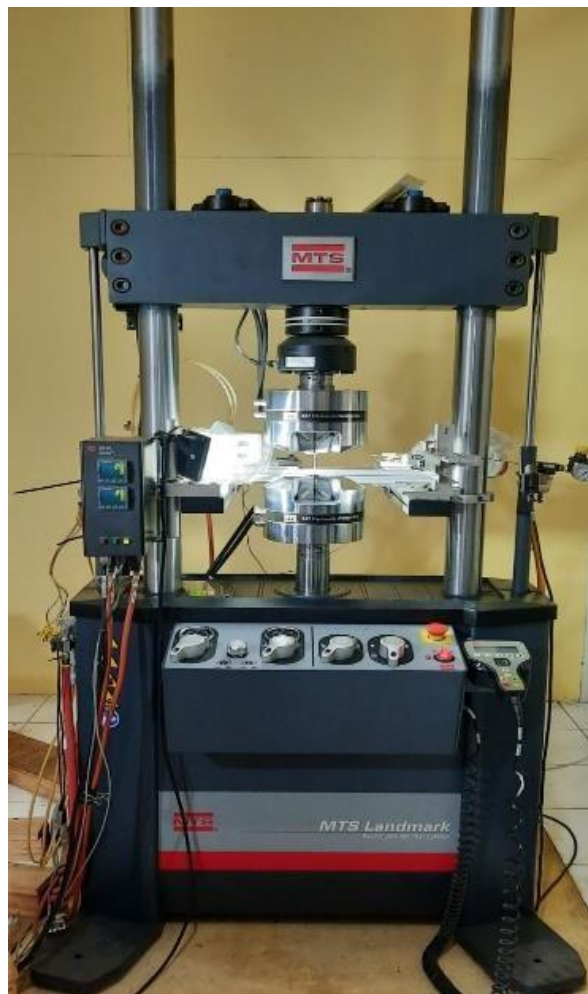
Gambar 15. Hydraulic servopulser mesin landmark MTS 100 kN.
