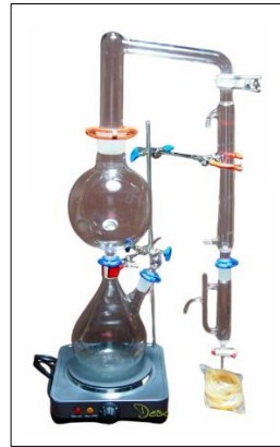
Gambar 2.9 Alat Destilasi Uap-Air (Andila et al. , 2020)
