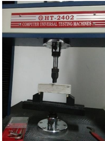
Gambar 4. Alat Uji Kuat Lentur Computer Universal Testing Machines
