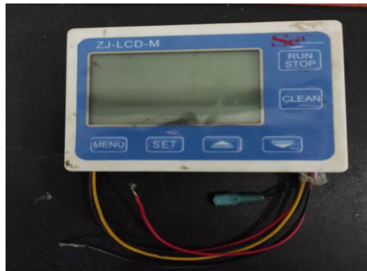
Gambar 3. 5 Water Flow Meter
