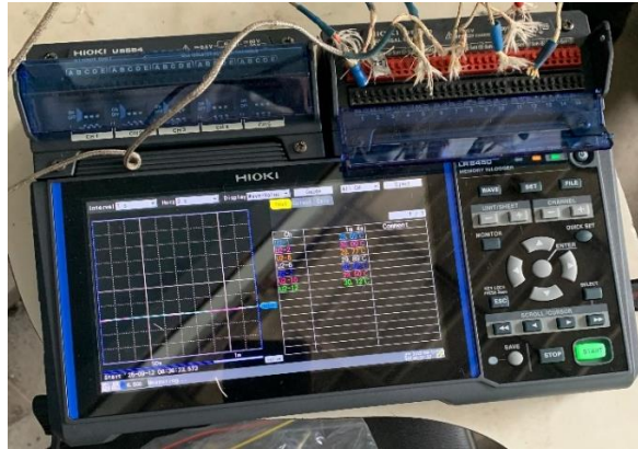
Gambar 3.3 12 Channel Temperature Recorder Datalogger
