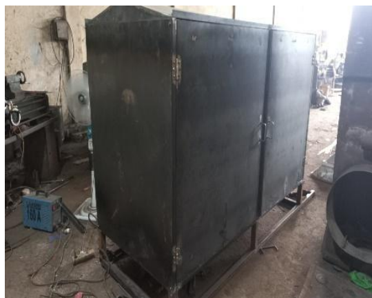
Gambar 3. 6 Finishing penempelan dinding bed dryer .
