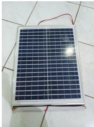
Gambar 3.7 Modul Surya 20Wp Polycrystalline
