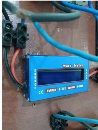
Gambar 3.15 Digital Watt Meter
