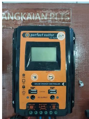
Gambar 3.13 Solar charge controller MPPT 70A
