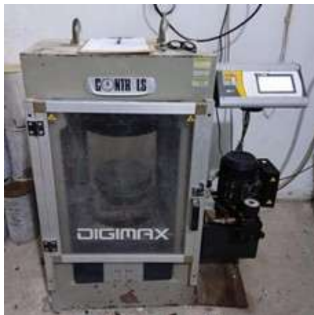
Gambar 3.13. Compression testing machine (CTM) .
