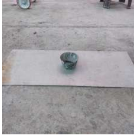
Gambar 3.12. Alat slump flow test .
